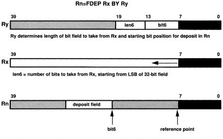
bit6 = starting bit position for deposit, referenced from LSB of 32-bit field Figure 2.6 Bit Field Deposit Instruction
