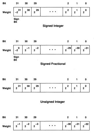
Unsigned Fractional Figure D.3 32-Bit Fixed-Point Formats
