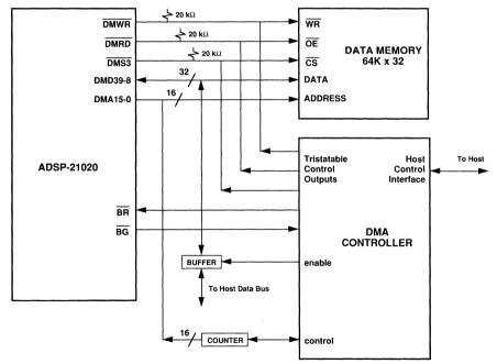
Figure 9.11 DMA Controller Interface Using Bus Request
