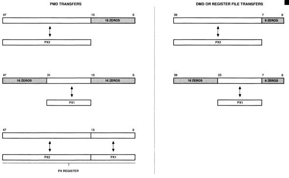
Figure 6.5 PX Register Transfers
