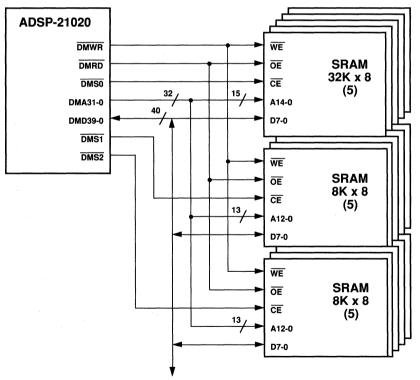
Figure 9.18 Memory Configuration with Unequal Capacitive Loads
