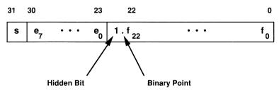
Figure D.1 IEEE 32-Bit Single-Precision Floating-Point Format
