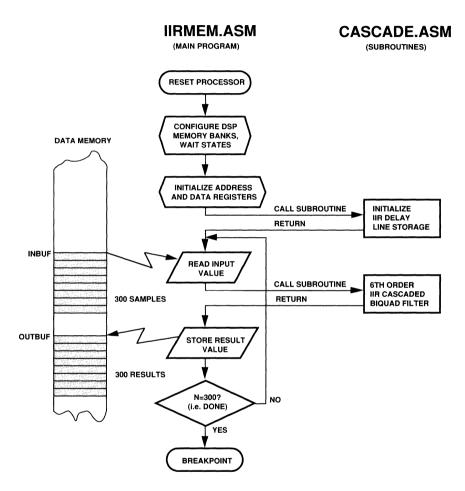
Memory-resident input sample vector ( "INBUF" ) is filtered, storing the result vector in another data buffer ( "OUTBUF" ). No interrupts are used. Execution ceases when done.
