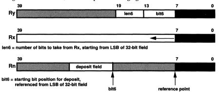
Example: If len6=14 and bit6=13, then the 14 bits of Rx are deposited in Rn bits 34-21 (of the 40-bit word).
