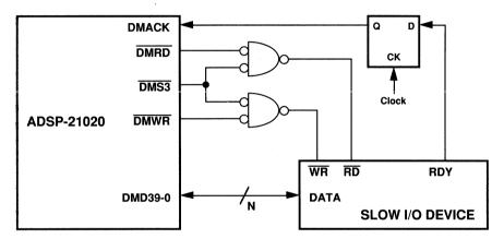
Figure 9.7 I/O Device Interface with Hardware Acknowledge
