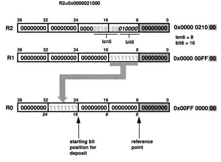
8 bits are taken from R1 and deposited in R0, starting at bit 16. ("Bit 16" is relative to reference point, the LSB of 32-bit integer field.)
