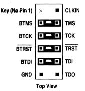
Figure 9.20 Target Board Connector For EZ-ICE Probe (jumpers in place)
