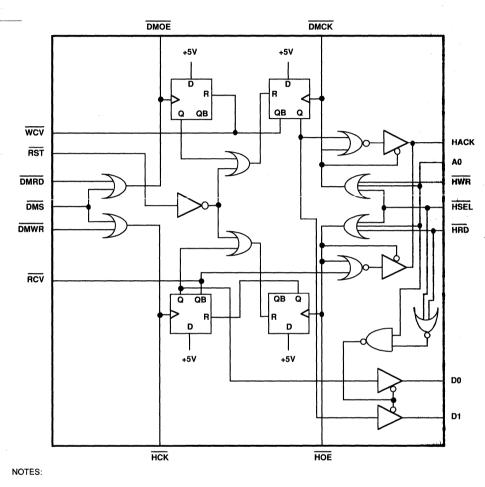
1. The latches shown are positive edge triggered D latches with asynchronous reset to 0.
