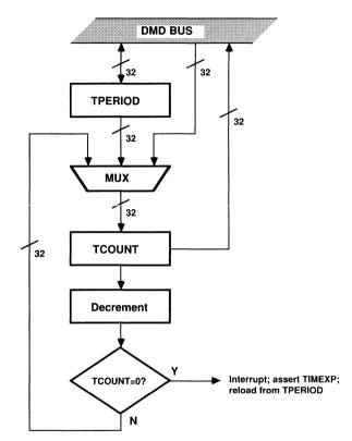
Figure 5.1 Timer Block Diagram
