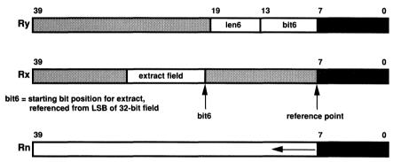
extracted bits placed in Rn, starting at LSB of 32-bit field
