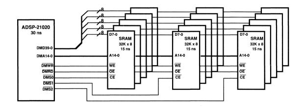
Figure 9.5 Interface to Three Data Memory Banks
