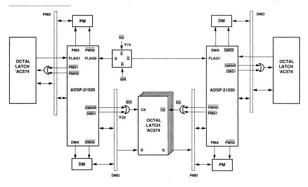
Figure 9.14 Serial Data Flow Using Buffers
