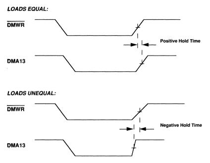
Figure 9.19 Effect of Unequal Capacitive Loads
