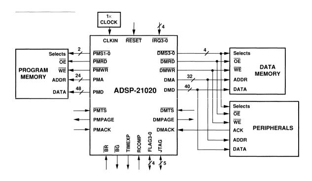
Figure 9.1 Basic ADSP-21020 System Configuration
