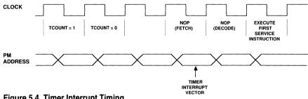
Figure 5.4 Timer Interrupt Timing
