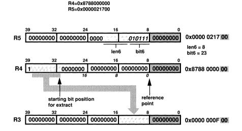
8 bits are extracted from R4 and placed in R3, aligned to the LSB of the 32-bit integer field.
