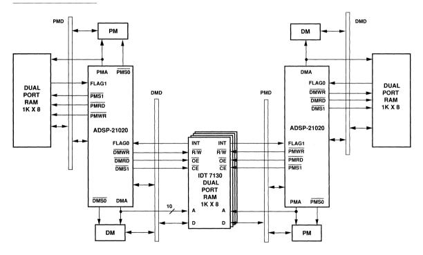
Figure 9.16 Serial Data Flow Using Dual-Port RAM
