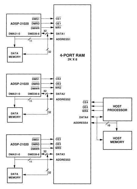
Figure 9.13 Four-Port RAM Configuration
