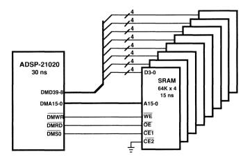
Figure 9.4 Interface to Single Data Memory Bank
