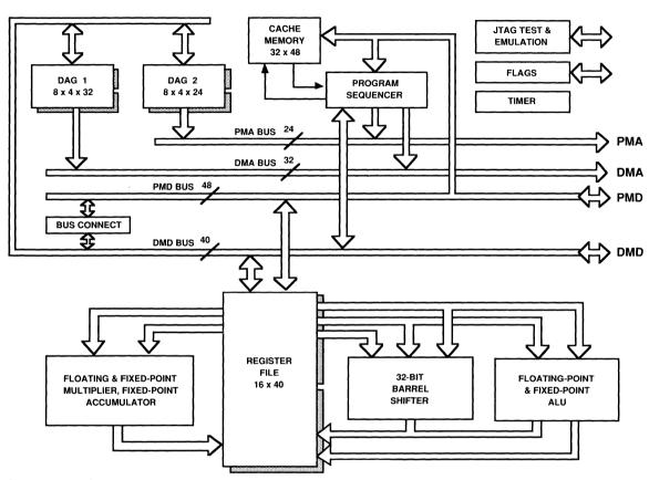
Figure 1.1 ADSP-21020 Block Diagram
