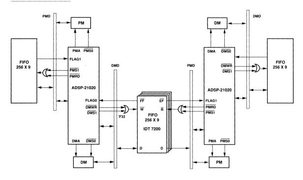
Figure 9.15 Serial Data Flow Using FIFOs
