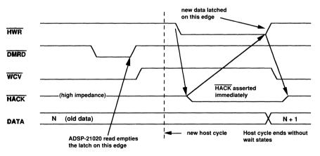
Figure 9.23 Host Write Timing
