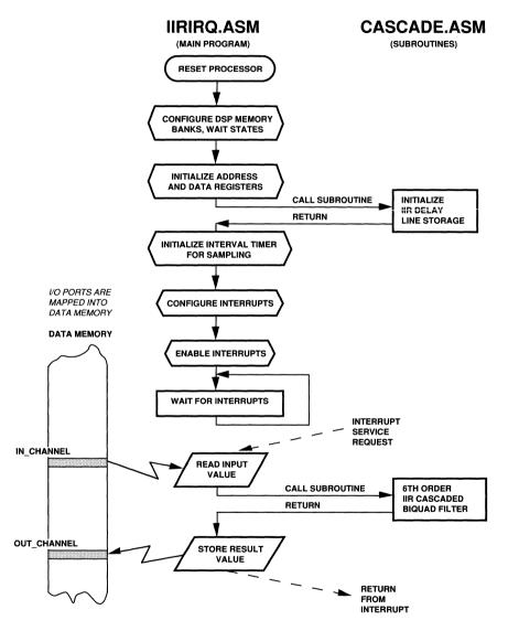
Sampled data is read from a memory-mapped I/O port during execution under interrupt control. Results are written out to another port. The DSP is interrupted at the sampling rate. The DSP's interval timer is the sampling clock.
