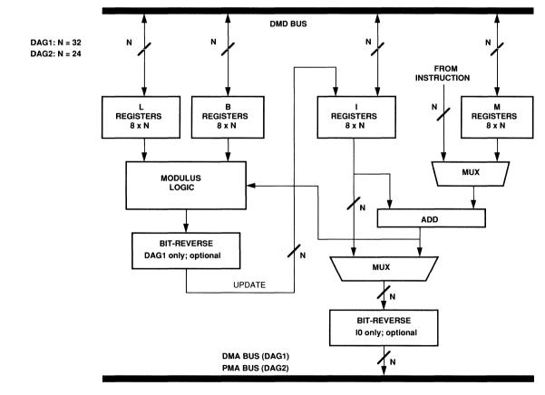
Figure 4.1 Data Address Generator Block Diagram
